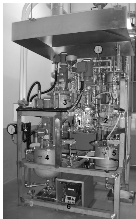
Fig. 5 Photo of bench-scale continuous-flow reaction system (1: reactor, 2: decanter, 3: mixing tank, 4: intermediate tank, 5: products tank, 6: feed pump).
